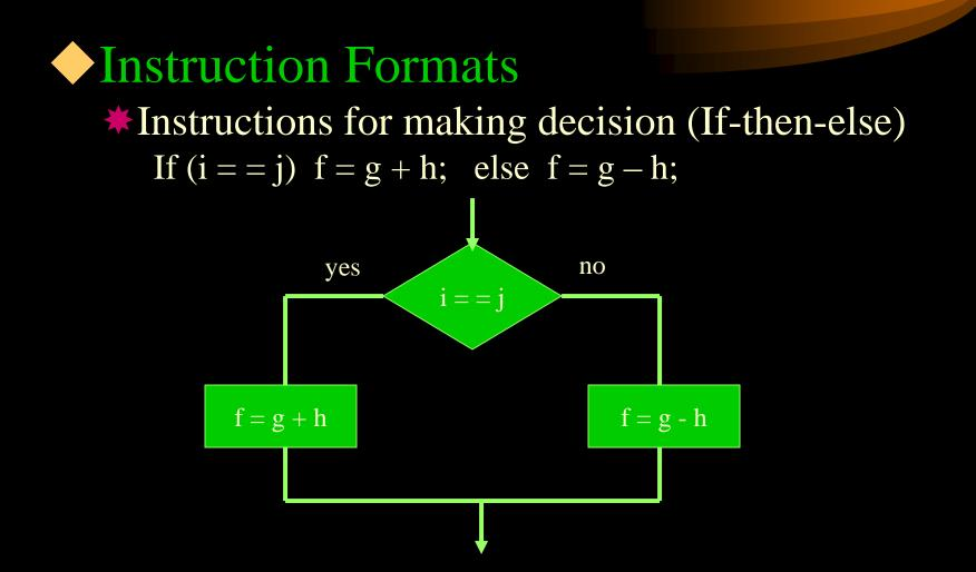
Instruction Formats **\*** If (i = = j) f = g + h; else f = g - h; \*Assuming *i* is in  $S_3$ , *j* is in  $S_4$ , *g* is in  $S_1$ , and h is in  $S_2$ . bne  $\$s_3$ ,  $\$s_4$ , Else goto Else if  $i \neq j$ add  $\$s_0, \$s_1, \$s_2$  f = g + hi Exit Else: Sub  $\$s_0, \$s_1, \$s_2$  f = g - hExit:
