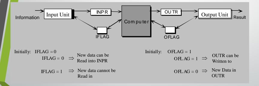
Input device: AA. If IFLAG =1 then goto AA. INPR  $\leftarrow$  "data", IFLAG $\leftarrow$ 1. Output Device: CC. If OFLAG =1 then goto CC. "data" ← OUTR, OFLAG←1.
